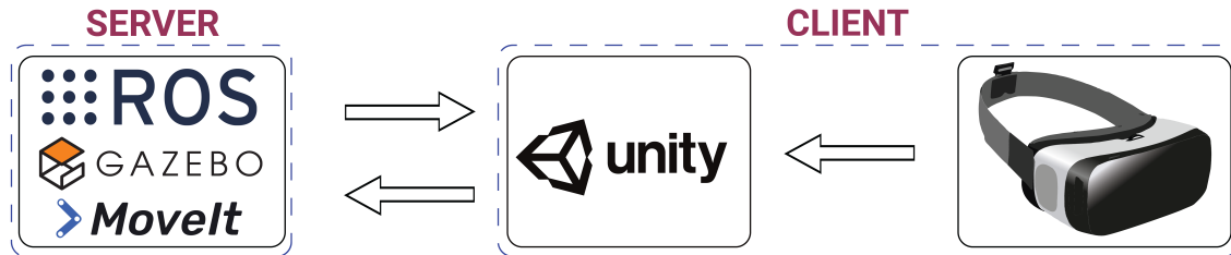
Figure 4: Evaluation testbed where: the Client executes a Unity-based simulation which the user interacts with through a VR headset; and the Server which receives information about objects on the workspace as well as user commands through ROS# which are processed by the Gazebo simulation engine and sent to MoveIt to prepare motion plans. The server and client can run on the same or different machines on different networks.
